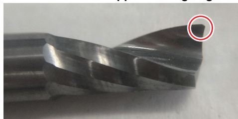
End mill with chipped cutting edge
