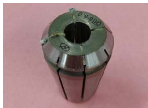
Debris accumulated in the chuck grooves
